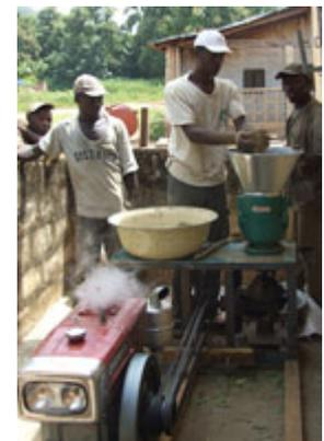
Figure 4 : *First use of the pelleting machine*
