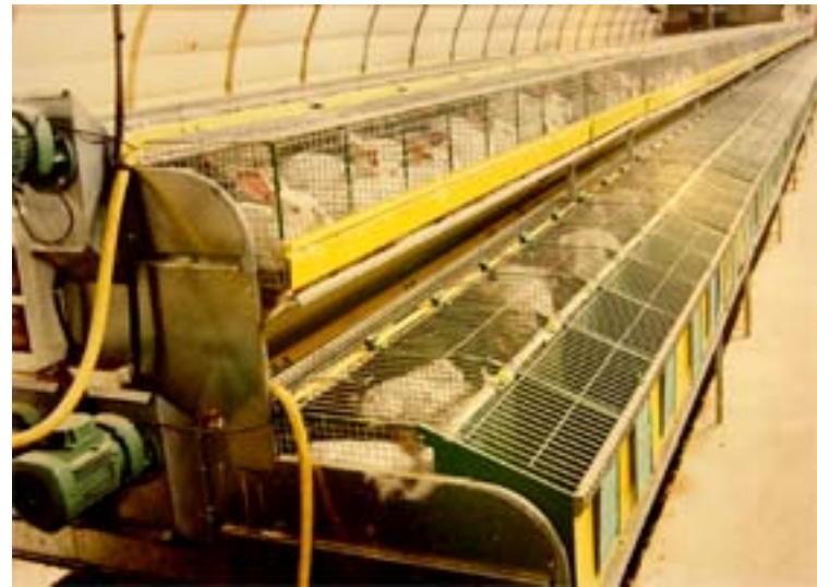
Feeding line could be long, but with no bend
